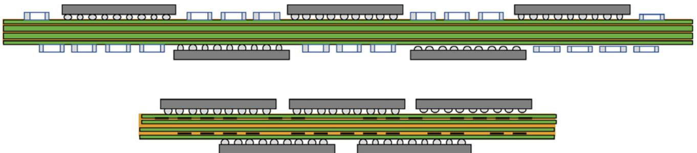
Figure 1: Comparing PCB area utilization of discrete surface-mounted resistors to that employing embedded thin-film resistors.
