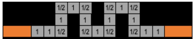
Figure 5: Serpentine resistor element design rules.
