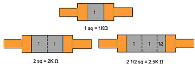
Figure 2: Basic “bar” resistor element design.
