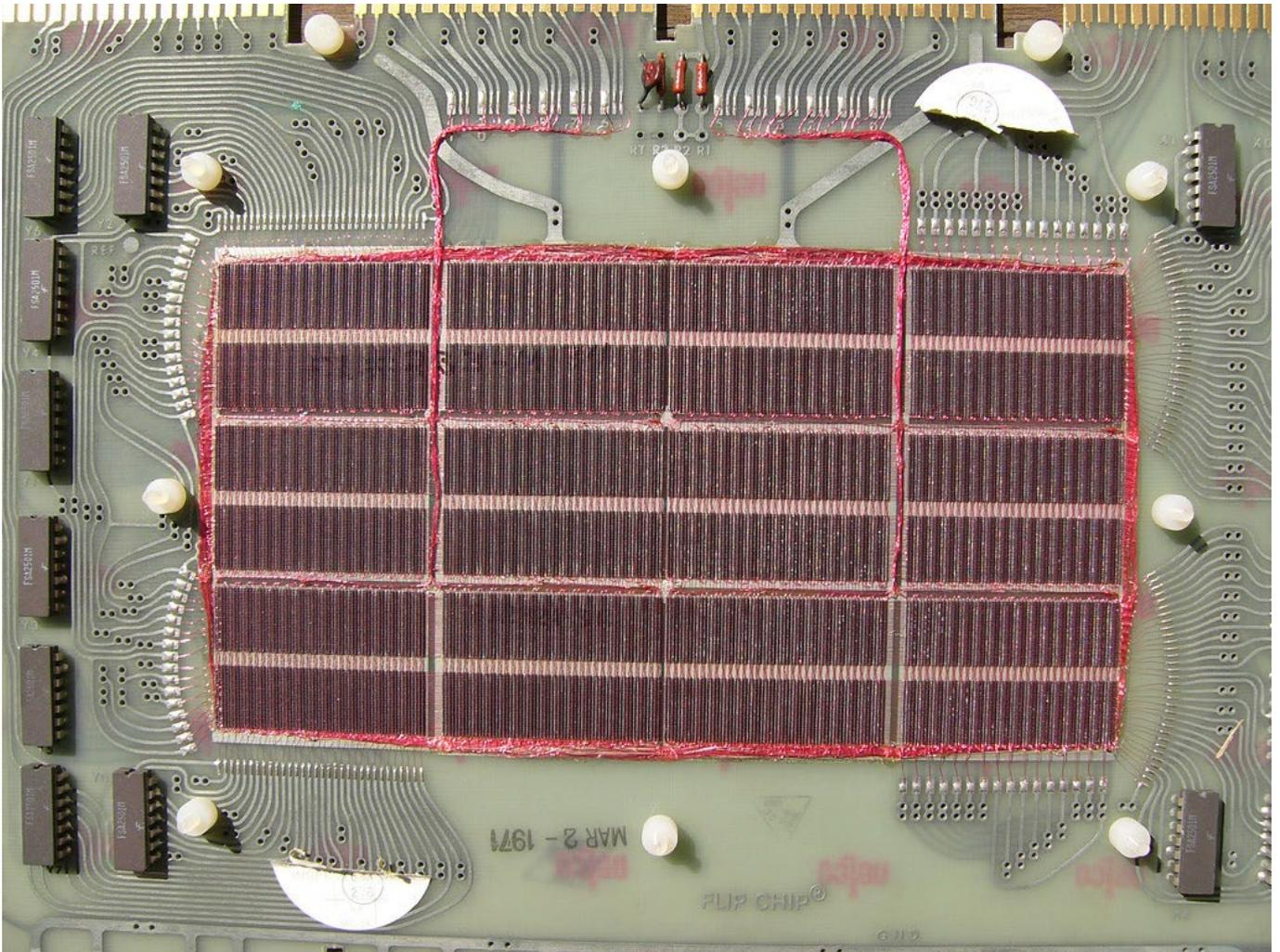
Figure 1: A 1970s core memory board.
