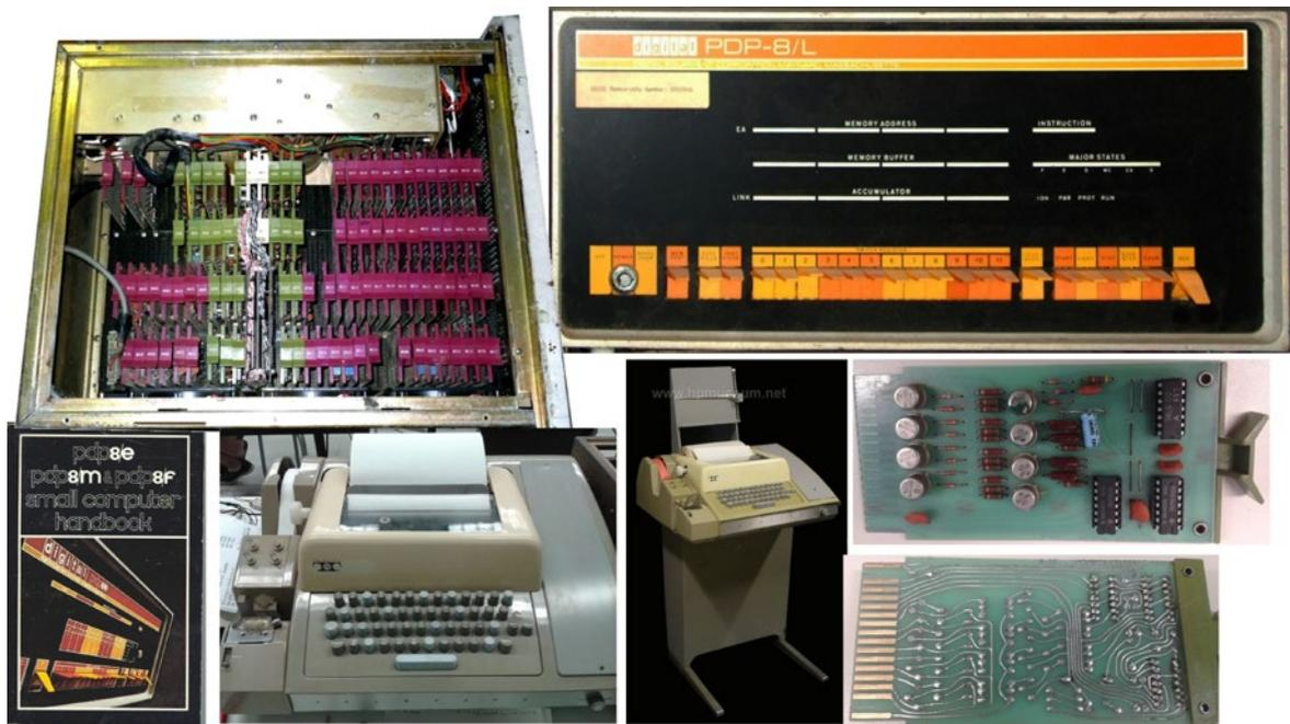
Figure 3: The digital PDP 8/L was the latest in 12-bit minicomputers. You had to manually toggle in the RIM Boot Loader with its front-panel switches so it could read a paper tape for the program from the ASR-35 teletypewriter. All the PCBs were single- and double-sided NPTHs with a wire-wrap backplane.
