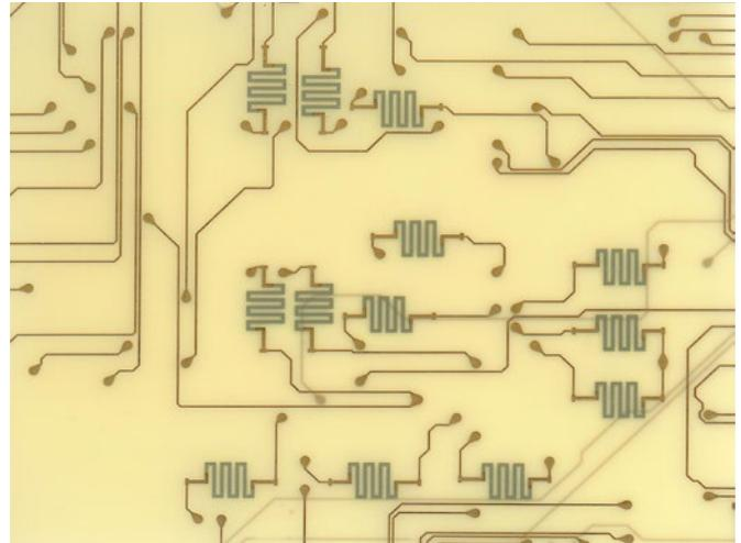
Figure 4: Serpentine-configured thin-film resistor examples. (Image source: Ohmega Technologies, Inc.)
