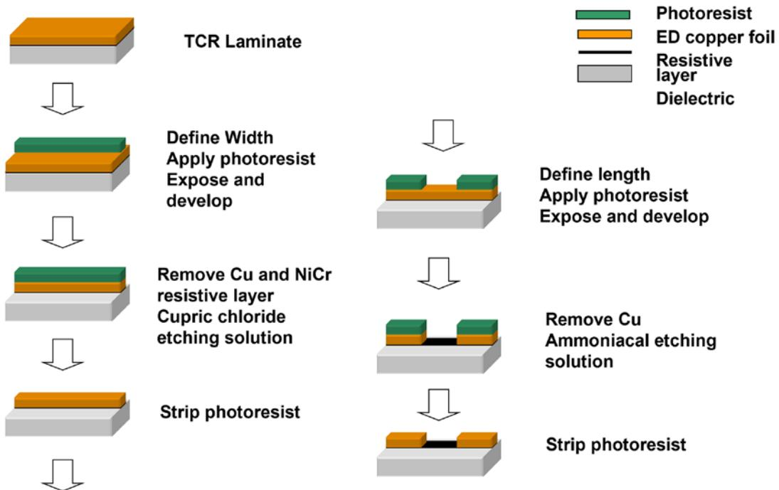
Figure 6: Thin-film resistor forming process sequence.
